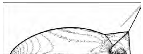
图 7 HCW-UL-Z, DMR 问题, 密度云图, 50 条等值线 Fig. 7 HCW-UL-Z, DMR problem, density contour, 50 levels
