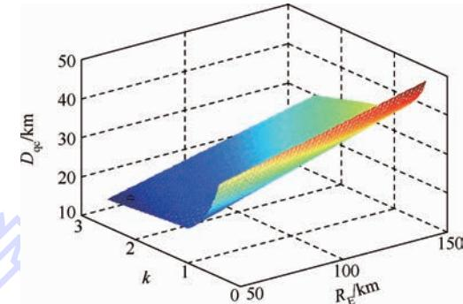
图 12  $k$ 、 $R_E$  与  $D_{qc}$  的关系Fig. 12 Relationships between  $k$ ,  $R_E$  and  $D_{qc}$
