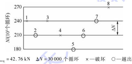
Fig. 3 Life up and down diagram
