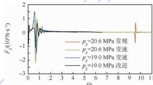
图 17 不同设计在  $n_z = 2.0$  工况下的作动筒力变化率对比Fig. 17 Actuator force derivative comparison of different designs ( $n_z = 2.0$ )表 8 不同设计在  $n_z = 2.0$  工况下的仿真结果对比Table 8 Simulation results ( $n_z = 2.0$ ) comparison of different designs
