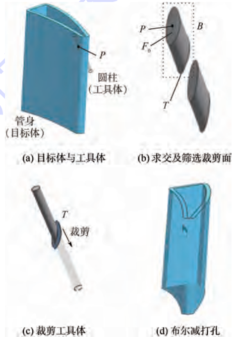
图9 截交包络裁剪法 Fig.9 Intersect-envelope trimming method
