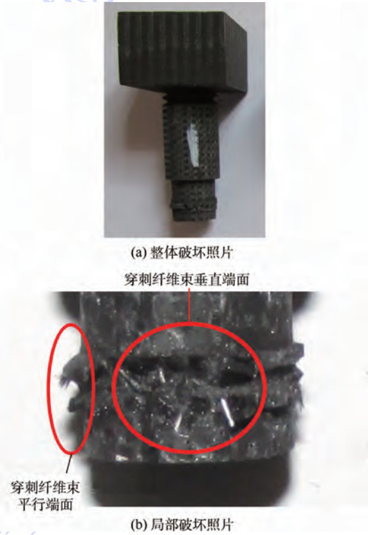
图 6 缎纹编织碳/碳复合材料单牙紧固件试验后照片 Fig.6 Photographs of satin weave carbon/carbon composite single thread fastener after test
