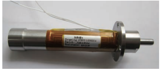
图 5 空间大载荷石蜡驱动器原理样机 Fig. 5 Principle prototype of large load space-used paraffin actuator
