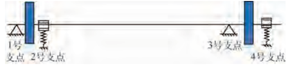
图6 采用支承松动设计的多支点柔性转子力学模型 Fig. 6 Mechanical model of multi-supported flexible rotor using bearing with loosening design
