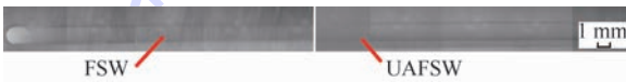
图 6 FSW 与 UAFSW 焊缝的 X 射线无损检测照片对比 Fig. 6 Comparison of X-ray nondestructive radiograms of FSW and UAFSW weld joints
