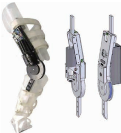
图 13 用于膝关节辅助运动的紧凑型串联弹性驱动器 [89] Fig. 13 Compact series elastic actuator designed for assisting knee joint motion [89]
