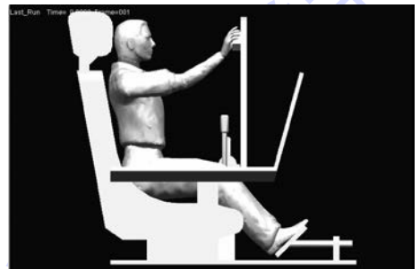
图 10 手握固定环下的飞行员动态响应仿真 Fig. 10 Simulation of pilot dynamic response as holding fixing rings
