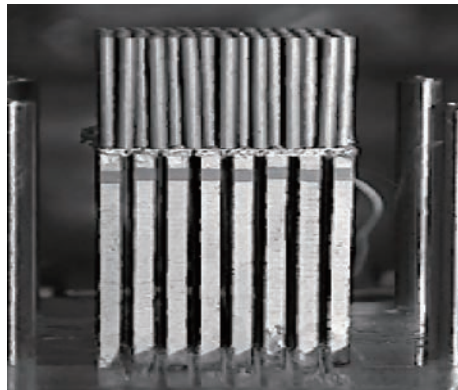
图3 Hayward表面触觉再现设备 [16] Fig.3 Surface tactile representation device by Hayward [16]
