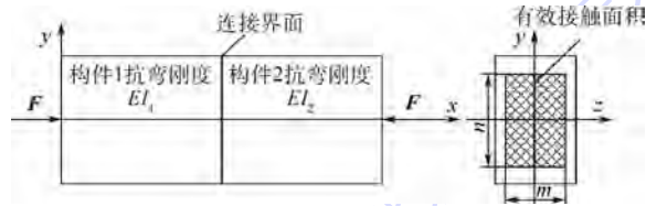
图3 连接界面有效接触面积示意图 Fig.3 Schematic of effective contact area of joint interface
