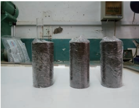
图 4 三瓣模成型土样 Fig. 4 Soil sample of three-section mould
