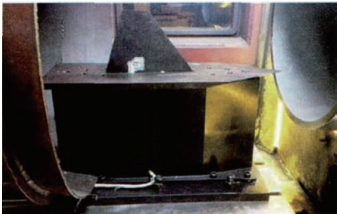
图 22 高超声速风洞中的翼面及颤振试验装置 [60] Fig. 22 Wing model and flutter testing apparatus in hypersonic wind tunnel [60]
