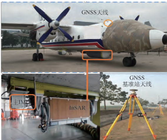
图 1 分布式 POS 与 InSAR 联合飞行实验的设备 Fig. 1 Flight experiment equipment with distributed POS and InSAR
