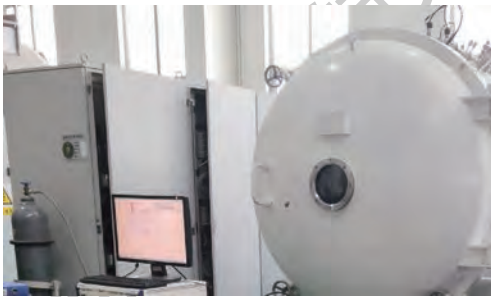
图8 0.5 kW级离子推力器性能测试设备 Fig. 8 Performance testing equipment for 0.5 kW class ion thruster
