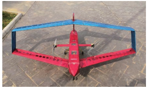
图 4 实验盒式倾转旋翼无人机示意图 Fig. 4 Schematic diagram of experimental box-wing tilt-rotor UAV
