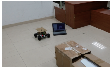
图 9 差分驱动轮式移动机器人及其实验场景 Fig. 9 Differential drive wheeled mobile robot and experimental scene
