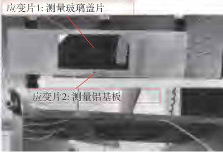
图 8 黏贴在铝基板上的空间太阳能电池三点弯曲试验示意图 Fig. 8 Schematic diagram of three-point bending test of space solar cells attached to aluminum substrate
